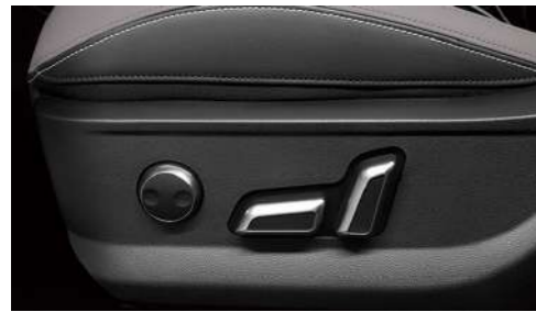
Driver 6 Way Power Adjustable Seat with 2 Way Power Adjustable Lumbar Support
